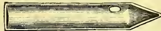
Glass tube for containing solutions for examination under the spectrum microscope. Half the real size. § 173.
